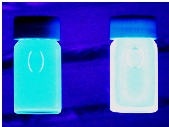
Fig. 5. The photographs of the fluorescence emission for poly( N -vinylcarbazole)-triethylborane complex (left; before F - addition) and poly( N -vinylcarbazole)/borate mixture (right; after F - addition).
